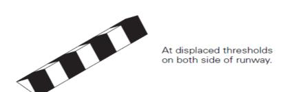
Black and white triangular box section marking displaced threshold.
